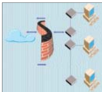
Packet filtering firewalls only look at the source and destination IP addresses of a packet, and then decide its fate
